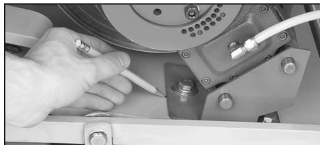
Figure 71. Marking caliper assembly location.
